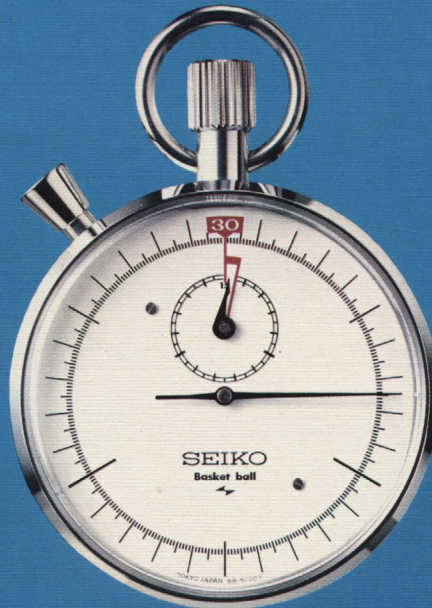
No. 63014 For basketball, 1/10 second, 15 minute accumulative recorder, 7j, all chrome plated, with neck cord.
